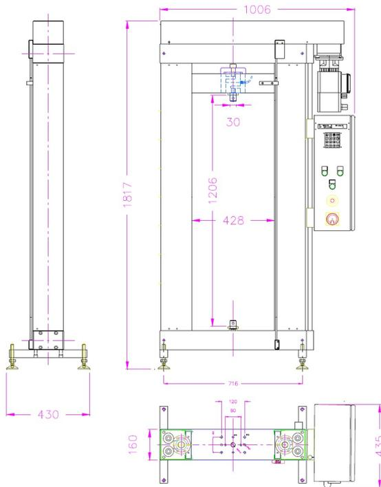
**Standmaschine 1200mm Hub**
